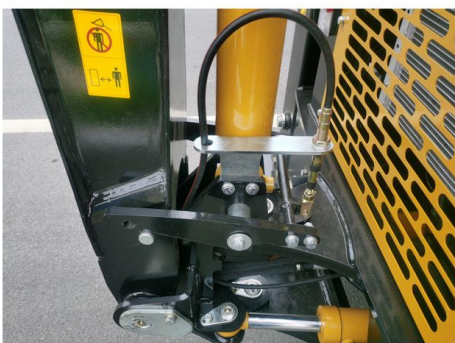
BACKHOE ARM LOCK
